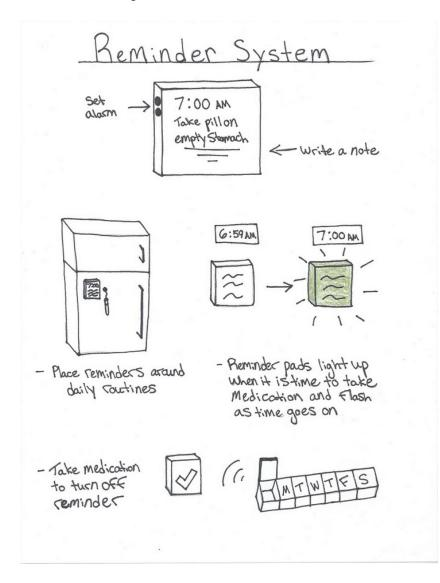
This is a portable system that allows users to place reminders around rituals and routines. Visual reminders are conveyed through text and ambient lighting cues. It is synced to the pill box which allows for many useful features including:
